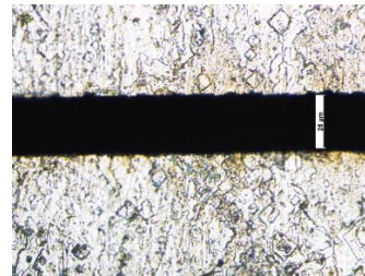
FIG. 2. Thin entrance slit width measured by a microscope
